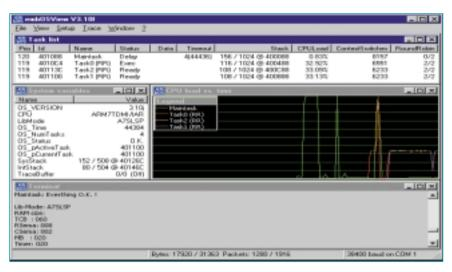
**embOS** is a real time operating system for embedded applications designed to offer the benefits of a fully featured multitasking system even for hard real time applications using minimal resources.
